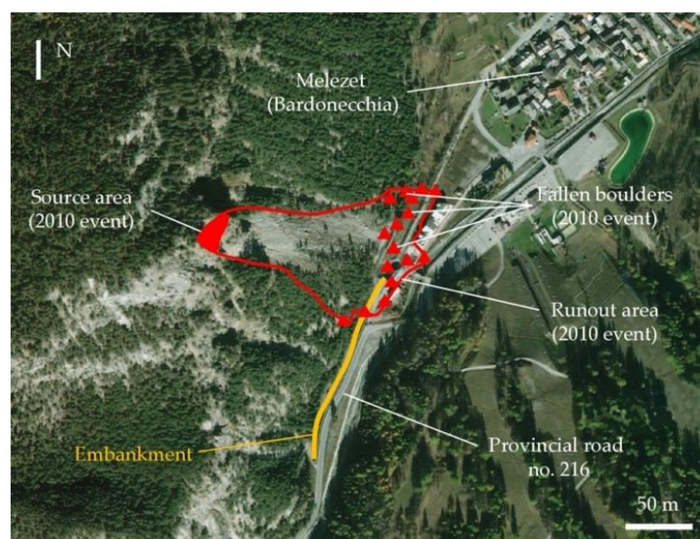
Figure 15. Map of the 2010 event. The red line highlights the runout area of the phenomenon and the red triangles define the location of the observed fallen blocks. The embankment (yellow line), located along the provincial road, was impacted by a cluster of boulders in the southern part of the runout zone.
