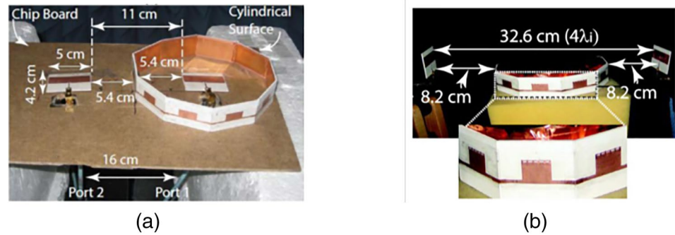
Figure 16. Cylindrical cloaking surface (a) interconnected 2-port microstrip (2-PM) (Jianfeng. Zhu et al., 2016) (b) interconnected 2-port reconfigurable microstrip (2-PFRM) (Naqvi et al., 2016).
