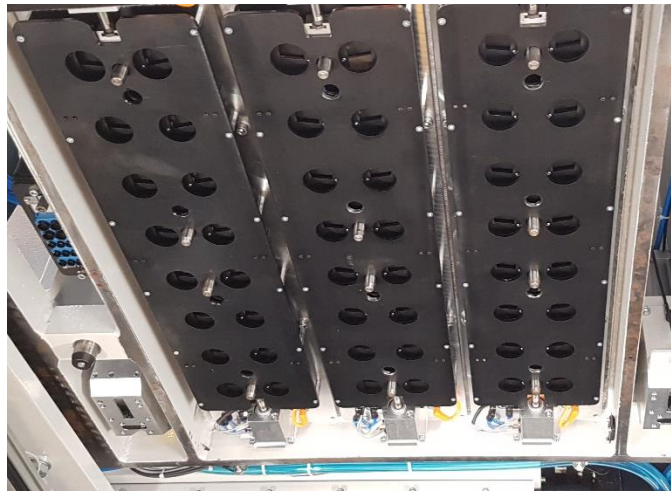
Figure 6-6 – Shutter placed between the exit of the sources and the optical fibers bundles
