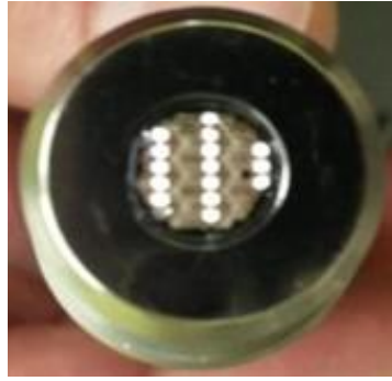
Figure 4-16 - Bundle 150 fibers output ferrule– Not randomized method
