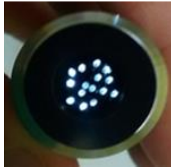
Figure 4-17- Bundle 150 fibers output ferrule–Randomized method
