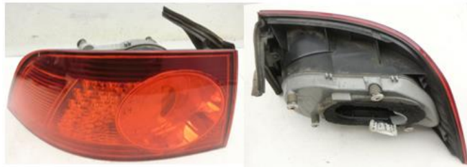
Figure 1-9 –Taillight: 1) lens in PMMA, laser transparent, 2) housing in ABS, laser absorbent
