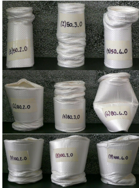
Fig. 17: Specimens at the end of the compression test.
