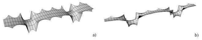
Figure 3: Form-finding of the Basento Bridge using simulated annealing: (a) with isotropic curvatures; (b) after reduction of transverse curvatures
