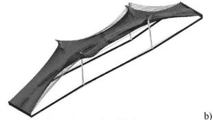
Figure 7: Stay-in-place, self-supporting formwork made of ferrocement. (a) setting-in-place by crane; (b) checking its buckling resistance
