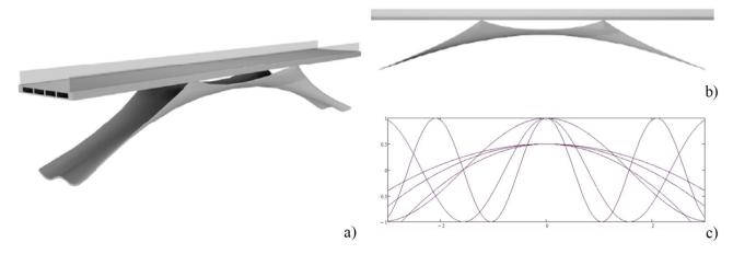
Figure 5: Shell-supported footbridge: (a) Perspective view; (b) lateral view; (c) parametric variation of the shell edge at the abutments to choose its optimum shape
