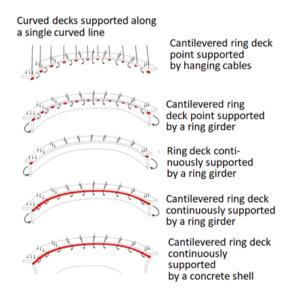
Figure 10: Curved cantilevered deck supported along a single curved
