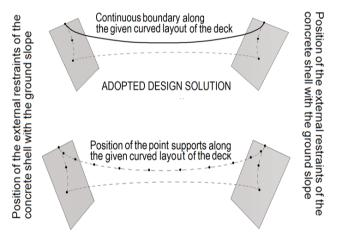
**Figure 11:** Assignment of the boundary conditions for the shell of a curved shell-supported bridge: (a) with the deck continuously supported by the shell top edge; (b) with the deck point-supported along the shell top edge
