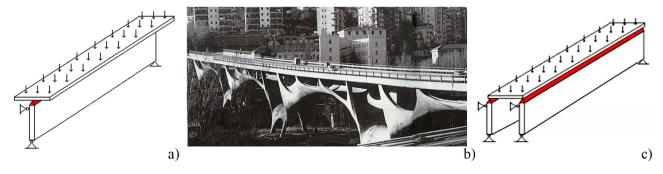
Figure 9: Unstable straight deck (a); Stable straight deck (b) and (c)
