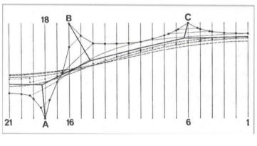
Figure 2: Form-finding of the Basento Bridge, (a) using soap bubbles; (b) integrating the membrane equation by finite differences (b)
