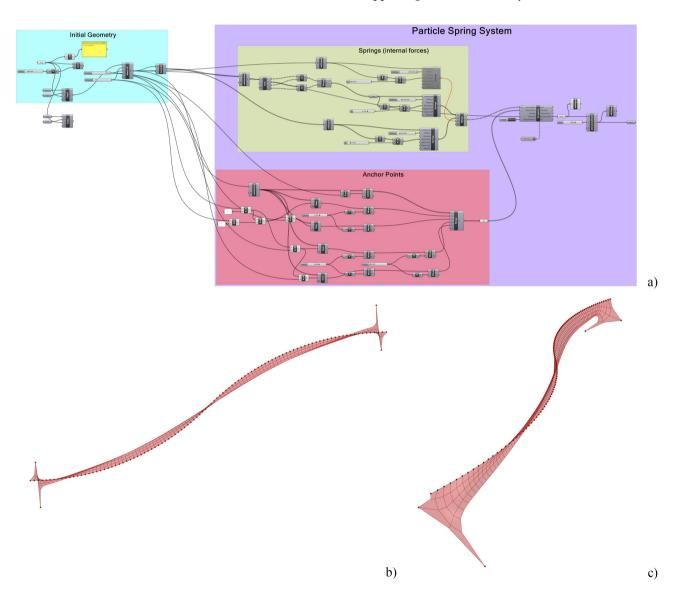
**Figure 16:** Form-finding by Particle-Spring System (PSS) of a S-curved curve and counter-curve shell: (a) Grasshopper/Kangaroo graphical form-finding algorithm; (b) top view of the optimal particle-spring network; (c) perspective view of the optimal particle-spring network
