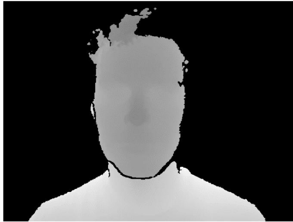
Figure 4.10 - Face detection: starting depth frame
