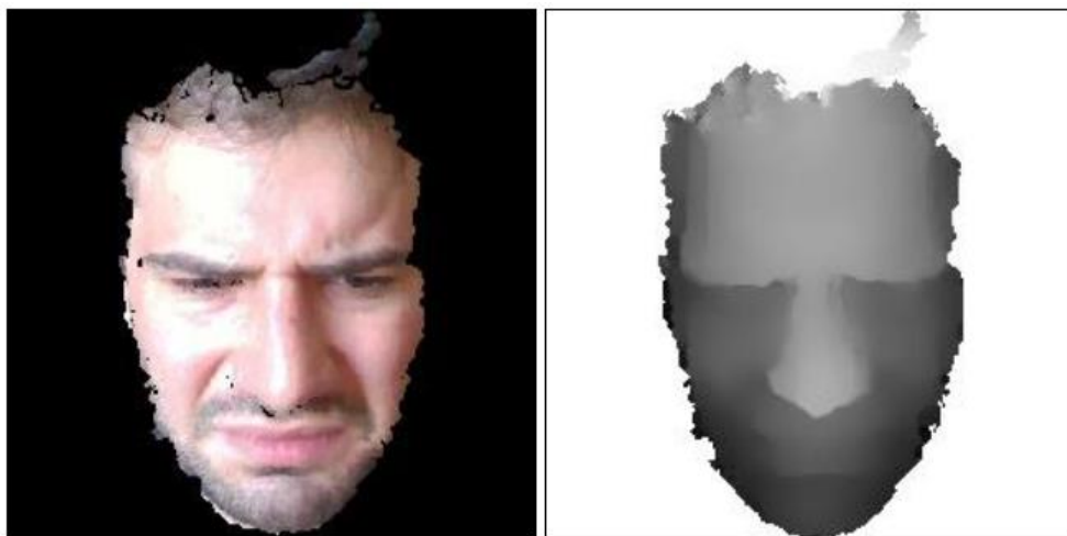
Figure 3.13 - Face oval detected in RGB (left) and Depth (right) frames
