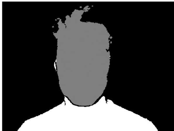
Figure 4.11 - Face detection: clustered depth frame
