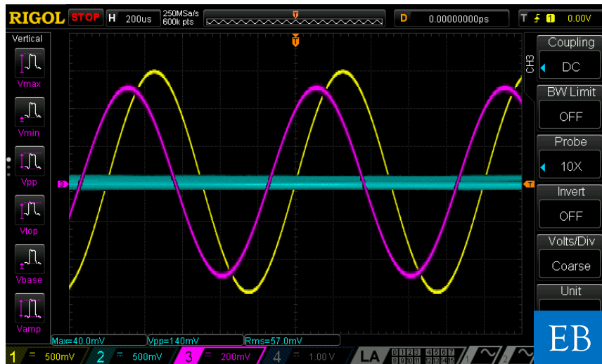
Figure 3.5.1. Example of input stress (yellow and pink curves) and output voltage (cyan line) for unfilled UV-cured EB at 150Hz.
