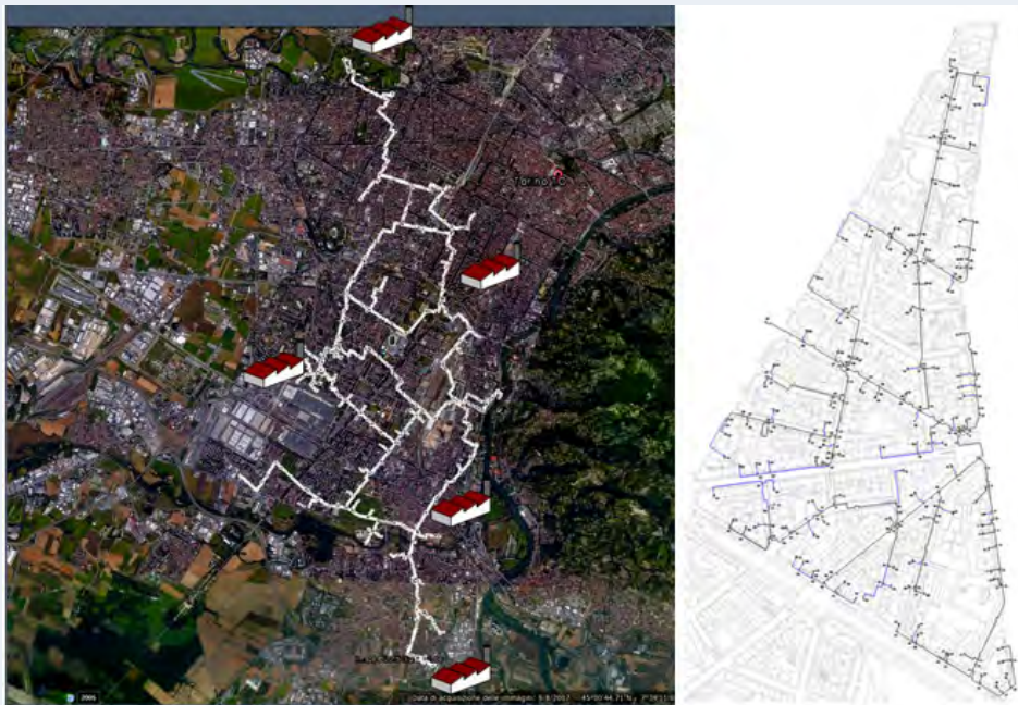
Figure 5: Transport network and distribution network
