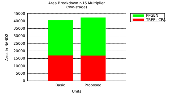
Fig. 9. Area breakdown for 2-stage pipelined multipliers.
