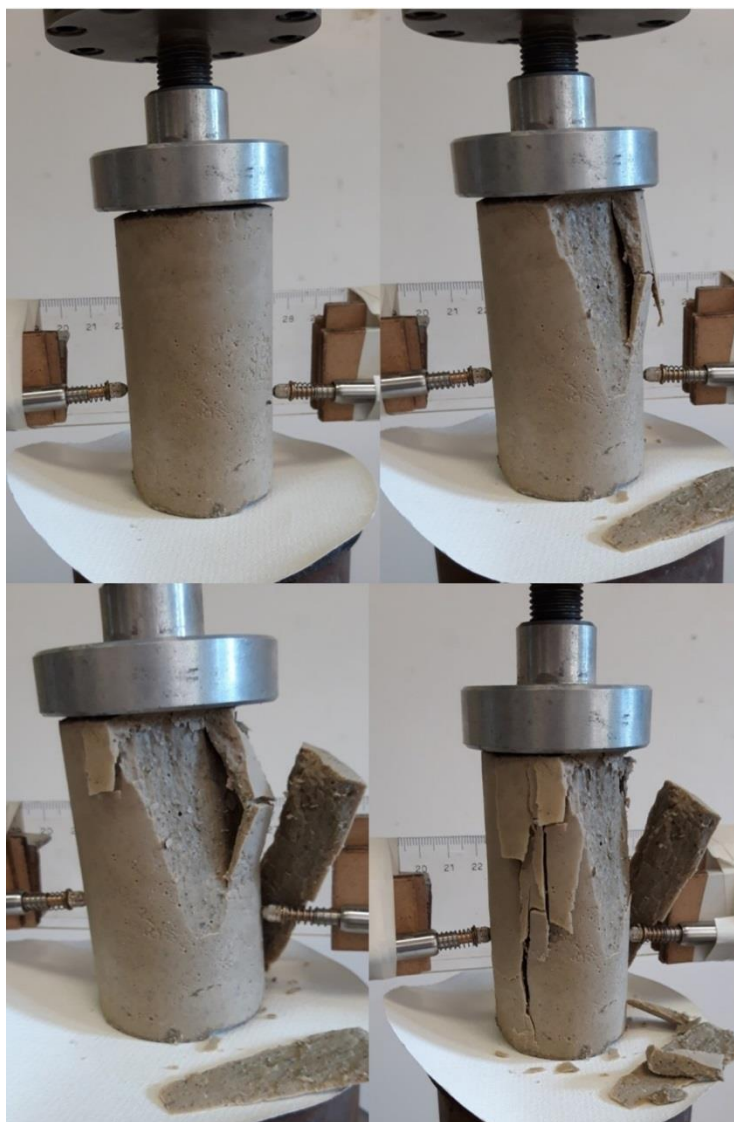
325 Fig. 6. Sequence of loading and failure after 28 days curing of the grout.
