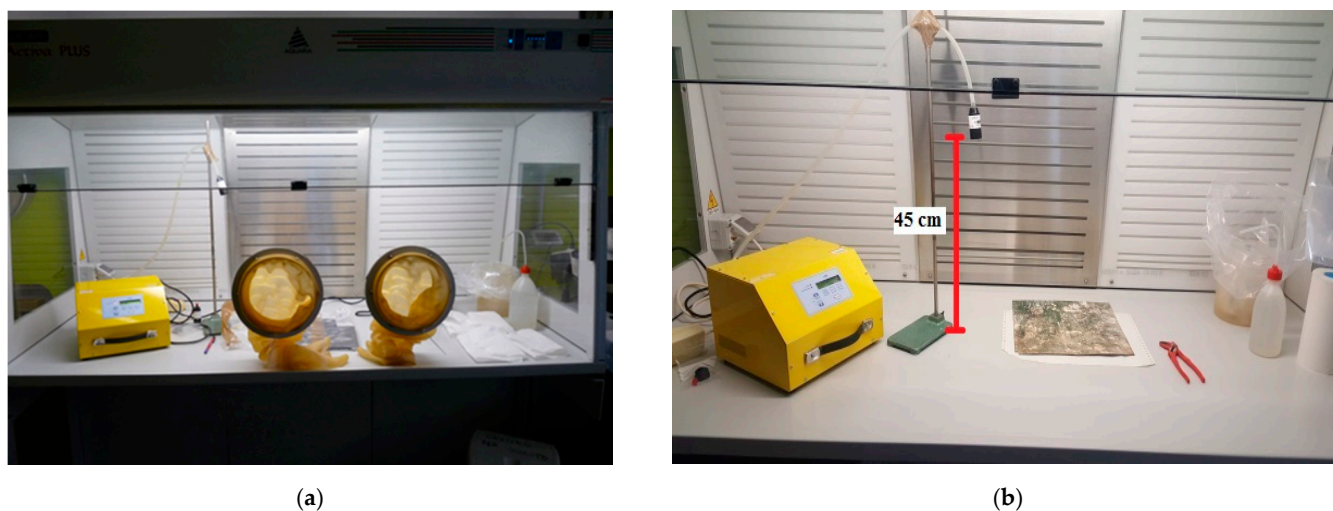
Figure 8. (a) Confined hood with gloves for simulation tests. (b) The airborne retrieval through a polycarbonate membrane.
