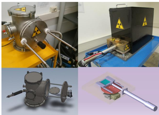
Figure 1. On the left: \alpha -irradiation system with a view of the inner sample-holder wheel. On the right: \beta -irradiation system and a scheme of its internal structure.
