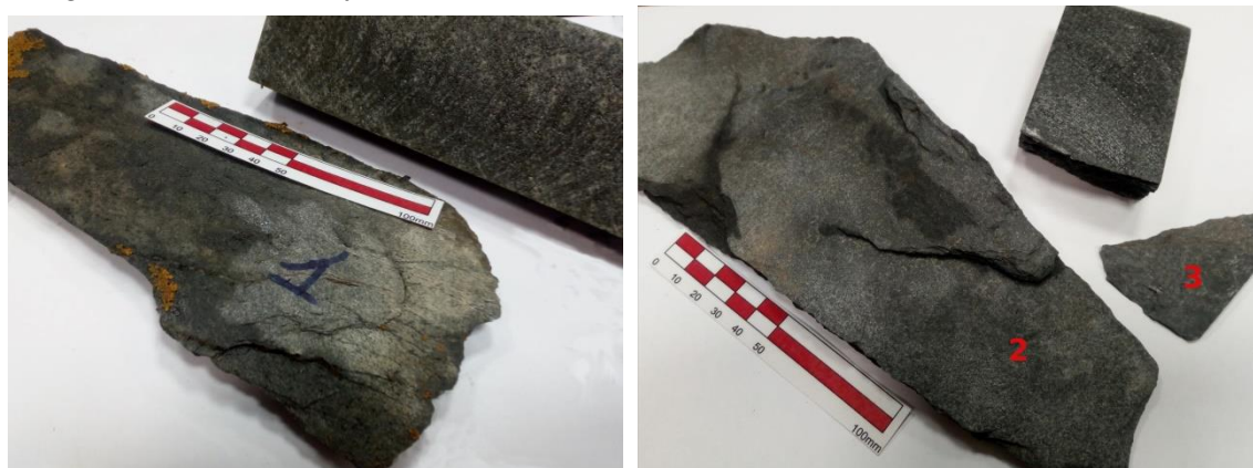
Figure 10. Comparison of sample from in situ and the laboratory specimens tested. On the left the sample 1 compared with Norway quartzite specimen; on the right samples 2 and 3 compared to Porfiroide specimen.
