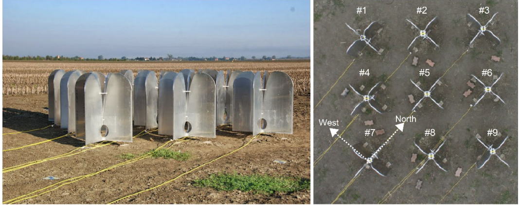
Fig. 1 – Pictures of MAD with optical fibers aligned in NS direction. Left: side-view. Right: aerial view (this figure has been processed to include cardinal directions and antenna labels).
