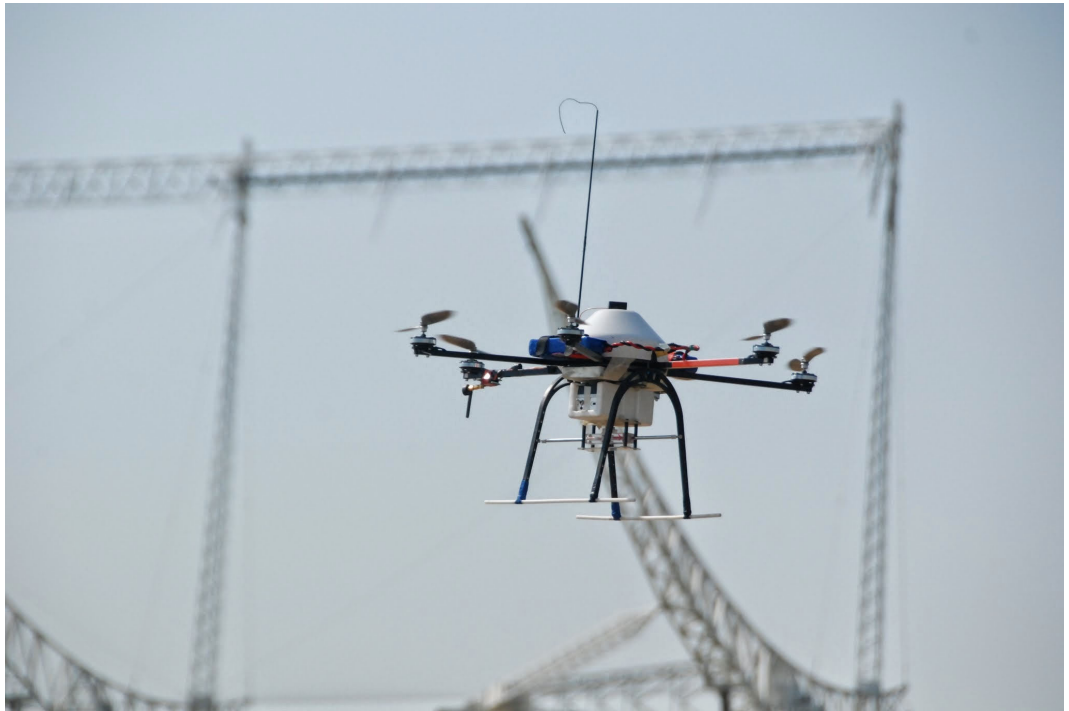
Fig. 2 – Foreground: hexacopter equipped with RF transmitter and telescopic dipole. Background: cylindrical reflector antenna of the Northern Cross Radio Telescope.
