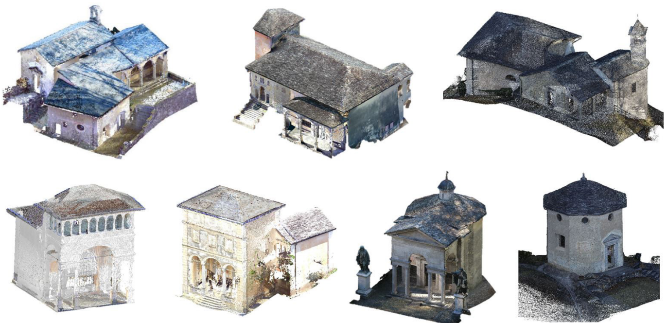
Fig. 6. Point clouds resulting from the integrated metric survey and obtained with different software.
