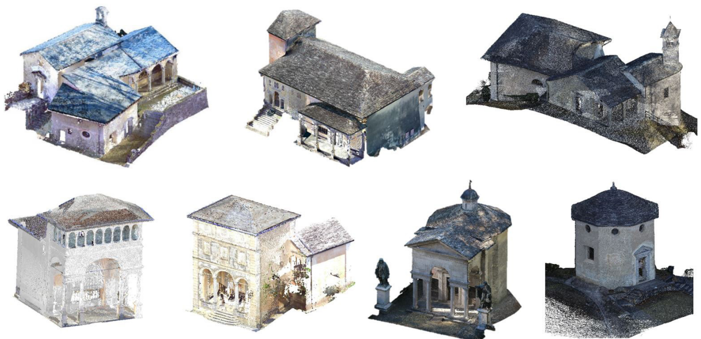
Fig. 6. Point clouds resulting from the integrated metric survey and obtained with different software.
