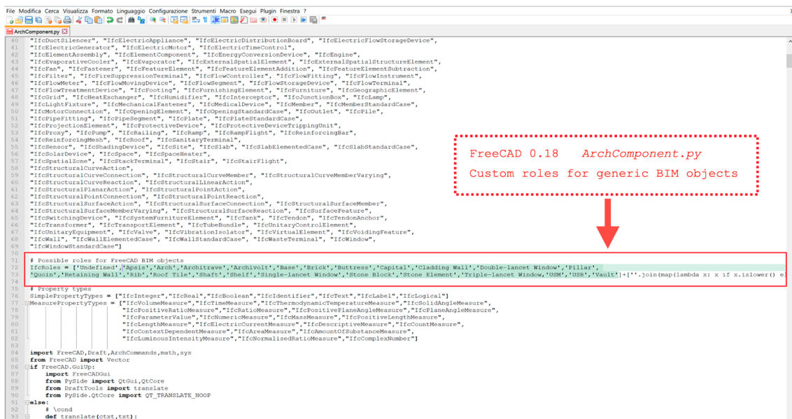
Figure 3. Access and modification of ArchComponent.py Python file by using FreeCAD 0.18: highlighted in green are customized and possible roles for BIM objects and related attributes below.
