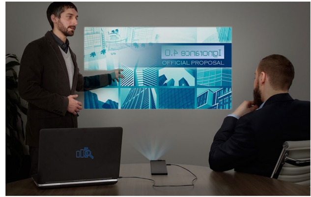
Fig. 1 Example of pocket projector, i.e., small hardware device designed to project content from a smartphone, camera, tablet, notebook or memory device onto a wall or other flat surface
