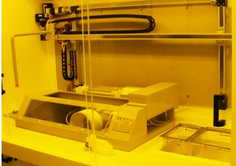
**Fig. 3** Automated ELO processing equipment developed at tf2-devices.
