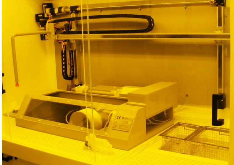
Fig. 3 Automated ELO processing equipment developed at tf2-devices.
