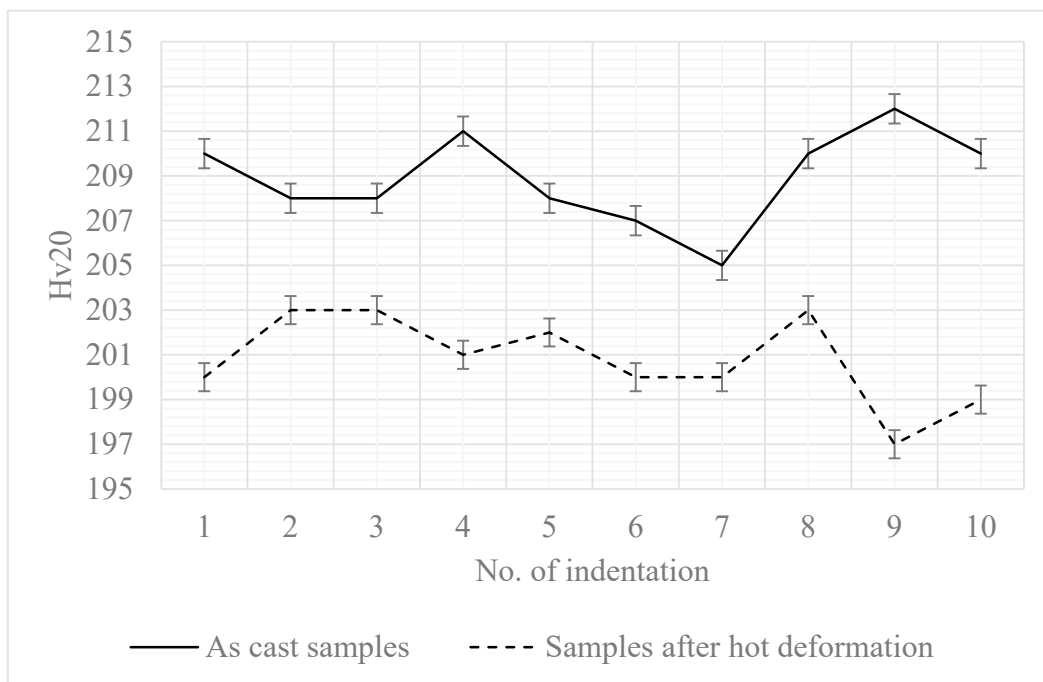
Fig. 3. Vickers hardness test results for the considered alloys.
