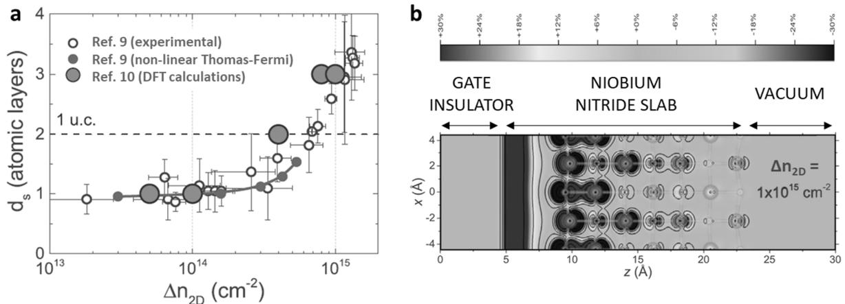
Figure 2: **a**, Number of atomic layers involved in the screening of the electric field, as a function of the induced charge density. **b**, Difference between the total charge density in doped and undoped NbN slab, sliced along the  $(x, z)$  plane. Grey-scale map is in linear scale between  $\pm 30\%$  of the maximum density difference in the accumulation layer. Adapted from Ref. 10.
