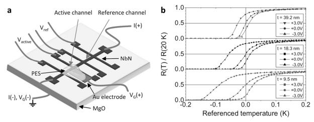
Figure 1: **a**, Sketch of a NbN-based EDL-FET in the dual channel configuration (active + reference). **b**, Normalized resistance of the active channel as a function of the temperature referenced to the midpoint of the ungated transition, for different applied gate voltages and film thicknesses. Adapted from Ref. 9.
