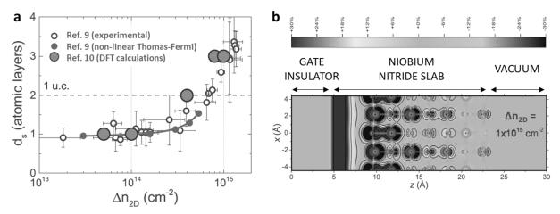
Figure 2: **a**, Number of atomic layers involved in the screening of the electric field, as a function of the induced charge density. **b**, Difference between the total charge density in doped and undoped NbN slab, sliced along the (x,z) plane. Grey-scale map is in linear scale between  $\pm 30\%$  of the maximum density difference in the accumulation layer. Adapted from Ref. 10.
