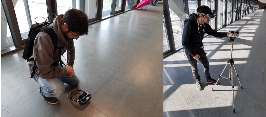
Fig. 3. Measurements of TA for the NOLO TM HMD (left) and controller (right).
