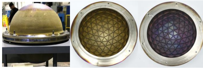
Fig. 14 Component after relevant environment testing: external and internal surfaces.
