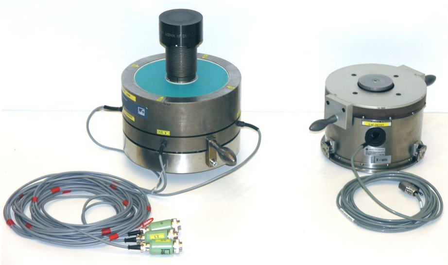
Figure 3: Photograph of the two 500 kN force transducers
