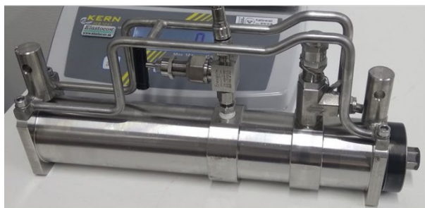
Fig. 3.5 The high-pressure dyeing vessel and its parts used in this work
