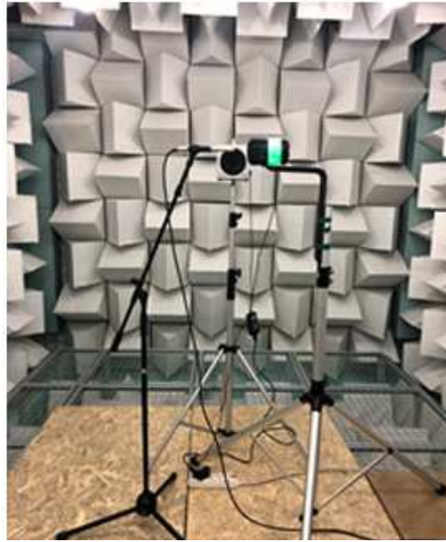
Figure 9. Set-up of the calibration by comparison in the anechoic chamber of PoliTo.
