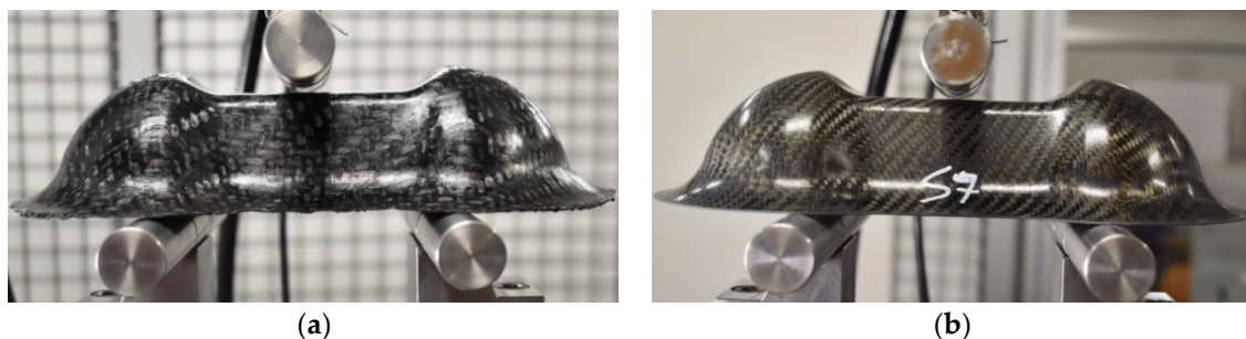
Figure 11. Double Dome specimens in GF/PP (a) and CF/EP-Solvay (b) before the bending test.
