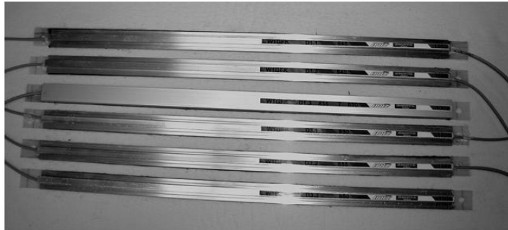
Fig. 15. The sensor pads for strain monitoring in the WT blade [74]
