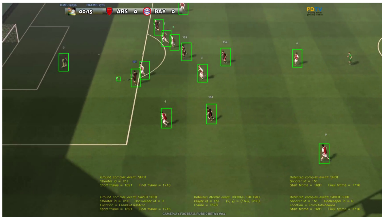
Fig. 6. Example of scene generated by the Gameplay Football engine, with superimposed ground truth bounding boxes and IDs of each player and the ball. The ground truth and detected events are also overlaid on the bottom of the scene: in this frame, a shot attempt is correctly detected.
