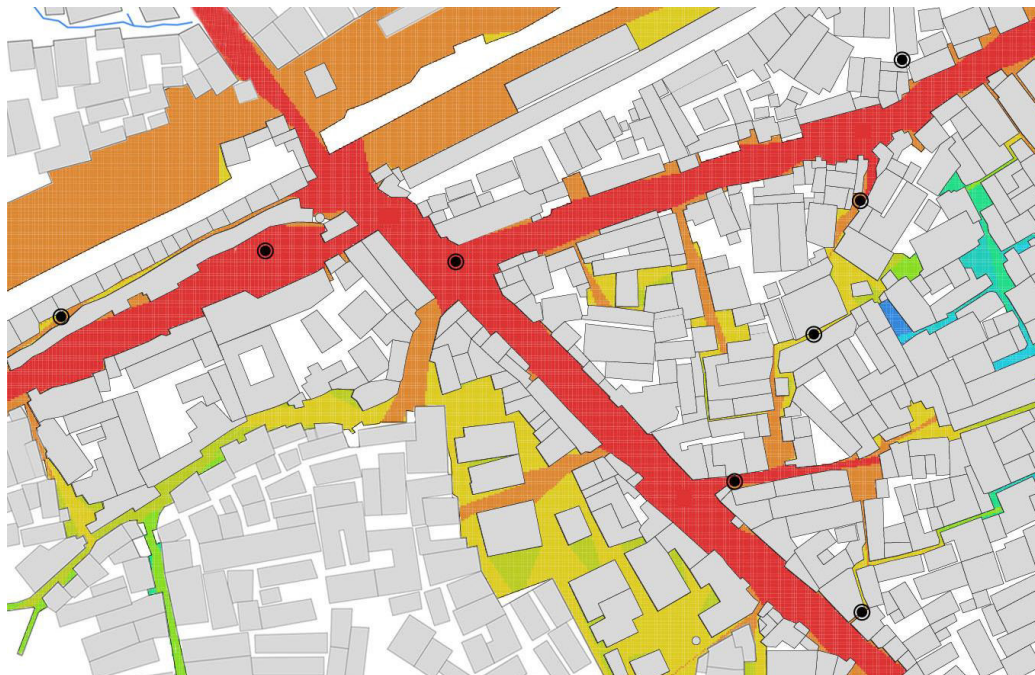
Figure 6, Step Depth analysis of the hot-spots in Kibera (Elaborated by the authors).
