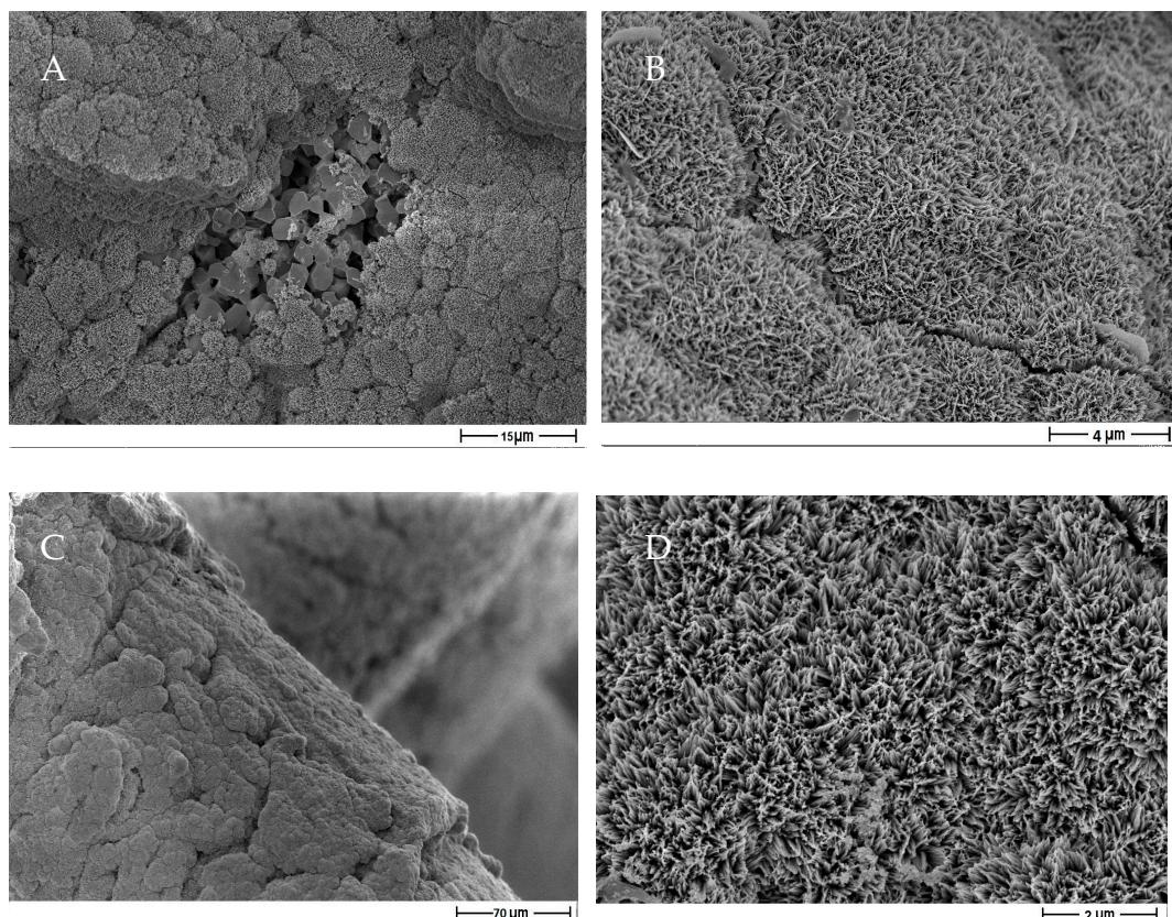
**Figure 13.** The new precipitated CaP layer on the surface of the bi-layer robocast structures. Low magnification images show the partial (**A**) and entire (**C**) coverage on the surface of dense and porous parts, respectively, and high magnification images show the evenly distributed rod-shaped crystals on the surface of the dense (**B**) and porous (**D**) parts.
