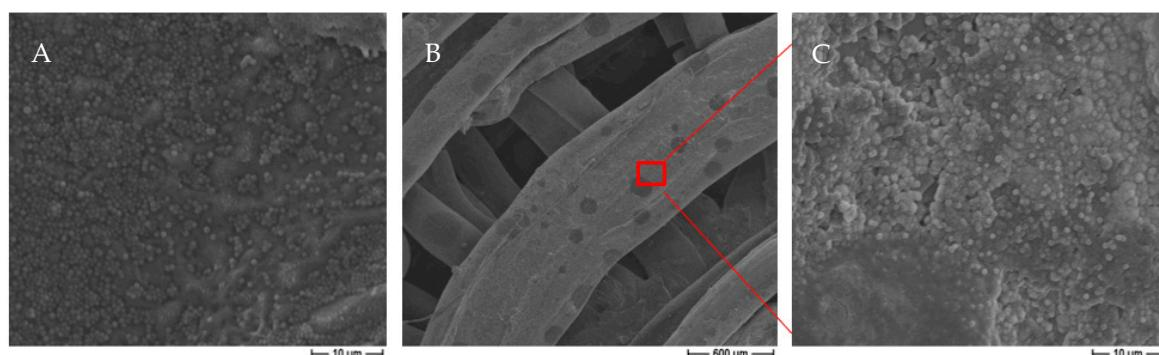
**Figure 16.** Micrographs of an  $\text{Ag}^+$ -free hybrid scaffold. (A,C) are high magnification of image (B): polymer (A) and ceramic (C) parts indicate bacterial biofilm on both surfaces.
