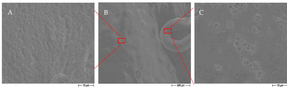
**Figure 17.** Micrographs of an  $\text{Ag}^+$ -functionalized hybrid scaffold. (A,C) are high magnification of image (B): polymer (A) and ceramic (C) parts indicate clean bacterial free surfaces.
