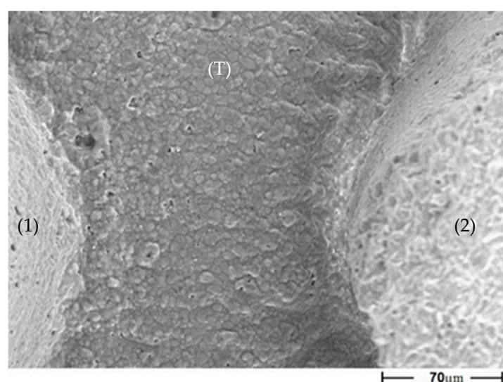
**Figure 4.** SEM image showing the contact area between interconnecting rods of adjacent layers.
