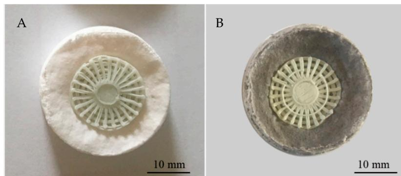
**Figure 14.** Digital photographs of two representative hybrid ceramic polymer samples. (A): Ag<sup>+</sup>-free PCL/BCP layer; (B): Ag<sup>+</sup>-added PCL/BCP layer.
