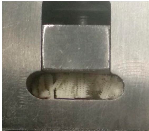
Figure 11. Remaining columnar parts of a collapsed 3D porous structure within the in-situ compression test device.
