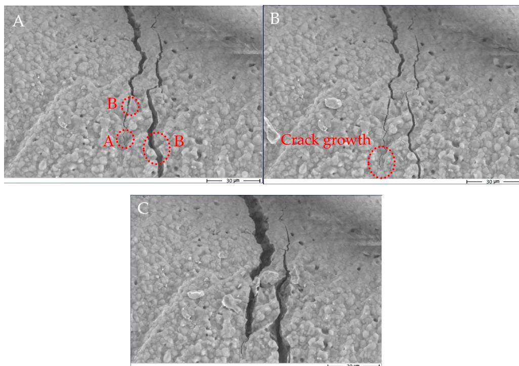
**Figure 12.** Cracks propagations through the microstructure of a porous sample under compressive loading taken by ESEM. (A) two parallel cracks propagated in opposite directions, (B) progression of the cracks tips by increasing the applied force, (C) condition of the cracks just before the final failure.
