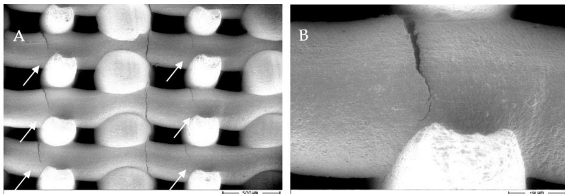
**Figure 10.** (A) Longitudinal cracks running through the structure of a porous scaffold during the compression test observed by ESEM, (B) a higher magnification image of a representative of the cracks.
