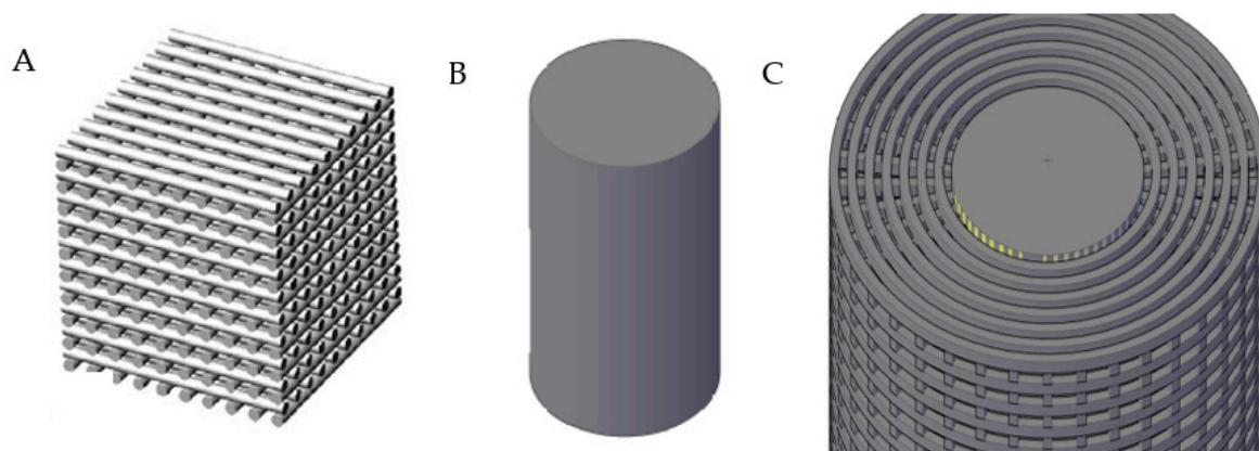
**Figure 1.** Schematic illustration of the 3D CAD designs for robocasting; lattice (A), dense (B) and bi-layer (C) models.
