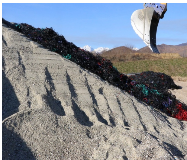
Fig. 2. Two types of non-conventional materials: the slope in the foreground is made of different fragmented and sieved glass; the bench in the background is made of polymeric cuttings from gasket production (credits Oggeri 2019).
