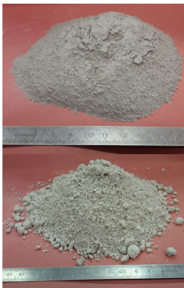
Fig. 5. Fine powder from quarrying/mining activities currently not recycled. (Top) from dry comminution process of olivine minerals. (Bottom) from wet comminution of quartz minerals (credits Oggeri 2019).
