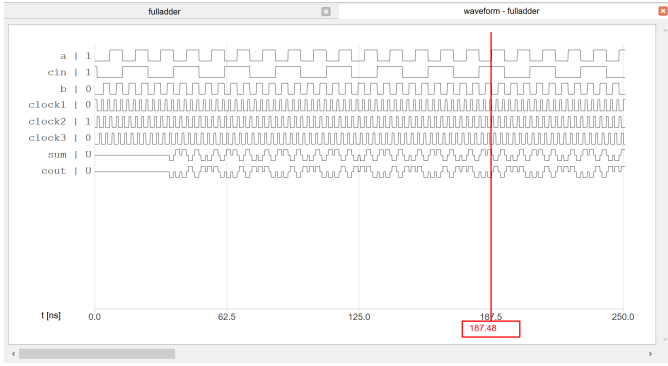
Fig. 6: Simulation waveforms of the full adder inside the ToPoliNano GUI.
