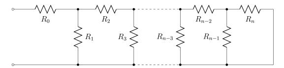
The equivalent resistance of this bipole,  $R_{eq}$ , can be expressed, and therefore calculated, as the continued fraction:
