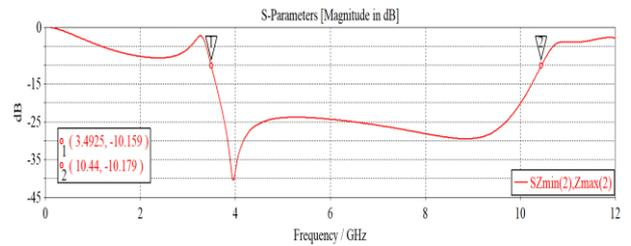
Fig. 13 Result for fig. 11 (wide-band) for TM polarization
