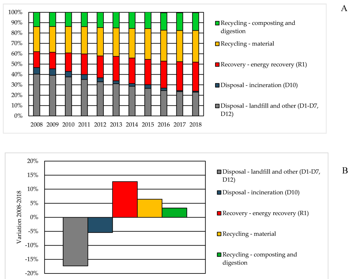
Figure 3. MSW management in EU-28 in 2008–2018: (A) historical evolution of waste management operations [1]; (B) net % variation of waste management operations between 2018 and 2008.
