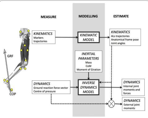
**Fig. 1** Schematic depiction of the workflow to estimate joint dynamics from measurements of kinematics and ground reaction forces (GRF), through kinematic and dynamic modelling of the body, and inertial parameters (inverse dynamics approach—IDA). The alternative estimation of external joint moments from kinematics and GRF is also reported
