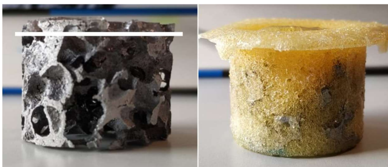
Figure 10. Aluminum open-cell foam sample (diameter 3 cm, the white line indicates the thickness of the cured superficial layer in the first experiment), and interpenetrating phase composite based on the impregnated and cured epoxy within the aluminum foam.
