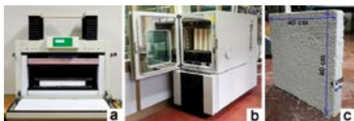
Figure 2 – a) The HFM apparatus for the thermal conductivity and specific heat capacity measurement; b) the climatic chamber adopted for the sample conditioning; c) sample size for the thermal conductivity and specific heat measurement
