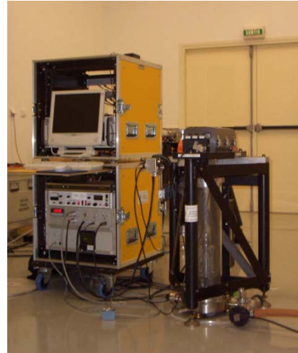
Fig. 1. Schematic drawing and picture of the IMG-02 absolute gravimeter.
