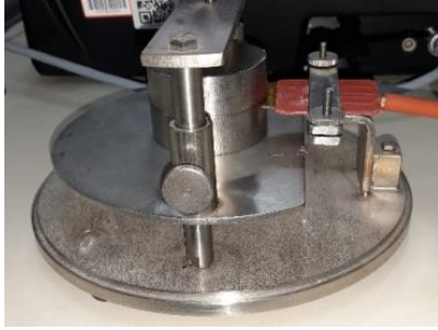
Figure 1. Typical assembly of samples and sensor
