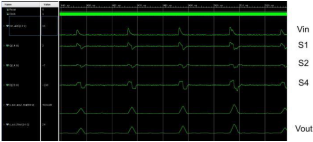
Figure 3. Signal waveform produced on the output of each stage
