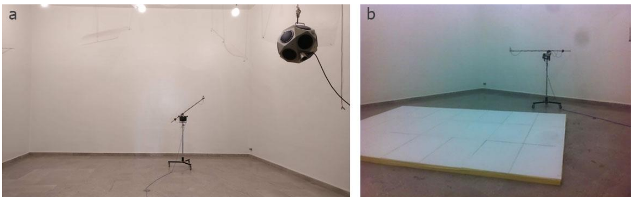
238 Fig. 3. Measurements in the full-scale reverberation room a) without and b) with the sample.
