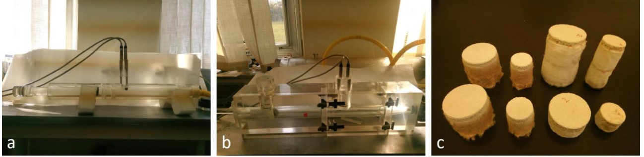
Fig. 2. Measurements set-up in the impedance tube with a diameter of a) 30 mm and b) 50 mm, and c) circular samples of the four materials with a diameter of 30 and 50 mm.
