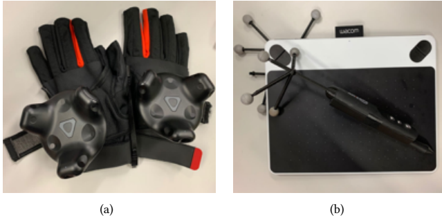
Figure 2: Hardware used in the formative study. (a) Manus VR gloves and HTC Vive trackers, (b) Wacom Intuos Draw digital tablet and pen, with buttons extracted from a slide presenter pen and OptiTrack M4 markers attached to a custom 3D printed case.
