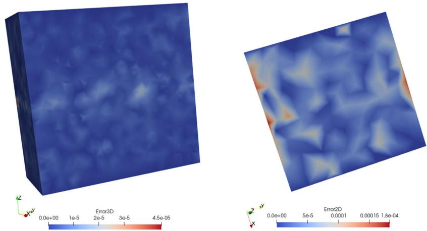
**Fig. 9** Problem 3: Computational domain, mesh and solution with the VEM on conforming meshes (left) and with the FEM based optimization method on non conforming meshes (right)
