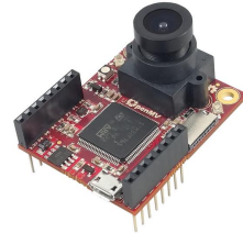
Figure 2. Deployment platform for the proposed solution. On a microcontroller platform (OpenMV Cam M7), we deploy a compact architecture made of about 100k parameters.
