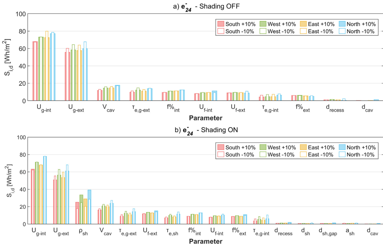
Fig. 9. S_{i,d} , Daily heat loss, Torino, all orientations, IDA ICE a) shading off b) shading on.
