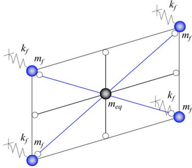
Figure 3. Reference scheme for the infilled frame model.
