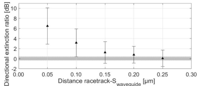
Fig. 4. Average and standard deviation of the directional extinction ratio as a function of the gap of couplers  $B_1$  and  $B_2$ , estimated over 20 simulations. The horizontal grey bar represents the value obtained without the S-shaped waveguide when CW and CCW fields have therefore the same power.
