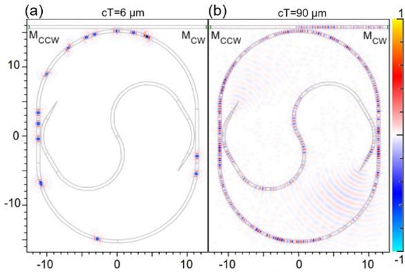
Fig. 2. Example of simulation for the device in Fig. 1a after (a) 6  $\mu\text{m}$  and (b) 90  $\mu\text{m}$  in unit of  $cT$ . The colours indicate the values of the field components perpendicular to the racetrack plane.
