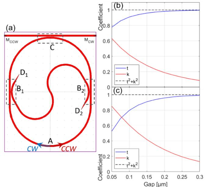
Fig. 1. (a) RSoft schematic of the considered racetrack and a S-shaped waveguide. (b,c) Coupling and transmission coefficients at  $\lambda=1.55 \mu\text{m}$  as a function of the coupler gap for the directional couplers  $B_1$  and  $B_2$  (b) and the directional coupler C (c).
