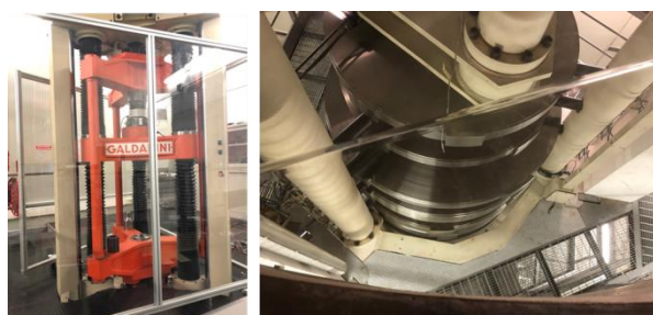
Figure 1: The 1 MN deadweight force standard machine
