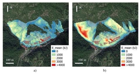
**Fig. 3** Output of the two forecasting analysis for the 5 m<sup>3</sup> scenario. The light grey area relates to the rockfall source zones characterized by the fractured rock face, the light red rectangles highlights the Rassa village while the red buildings are the structures interested by the 2018 event: a) Rockyfor3D simulation, b) QPROTO simulation.
