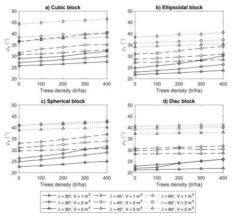
**Fig. 2** Energy line angle values sorted with reference to the block shape. a) Cubic shape gives the higher values of  $\varphi_p$ . b) and c) are related to ellipsoidal and spherical blocks, respectively. It can be seen that the corresponding angle are generally lower in this case because of the higher rotational inertia of these shapes. d) In disc shape case the minimum angles are obtained.
